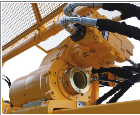
Powerful rotation unit 600 mt drilling capacity with NWL drill rod.
